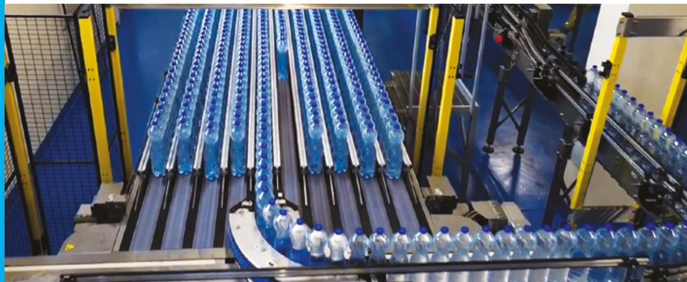
➤ **SYSTÈME SYNCHRONISÉ POUR L'EMBALLAGE SECONDAIRE ET TERTIAIRE COMPOSÉ DE: DIVISEUR DV 500 ERGON + CONVOYEURS + FARDELEUSE SK 502 F ERGON + PALETTISEUR APS 3090 P SX ERGON**
