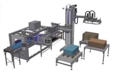
movements along the cross beam; an articulated arm based on SCARA technology that performs both vertical and horizontal movements for feeding the empty pallets and inserting the interlayers.
